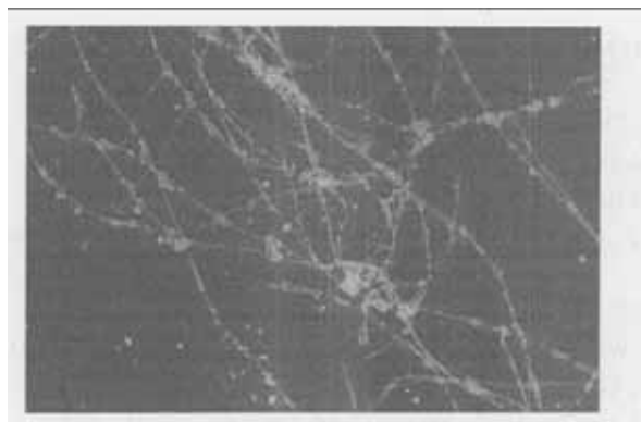
Fig. 5 Fluorescence micrograph of fibrilla morphology of 16-3 deposited from aqueous solution on cover glass with magnification of 100
