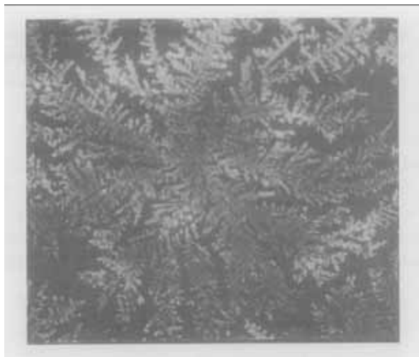
Fig. 6 Fluorescence micrograph of fractal-like morphology of 16-4 deposited from aqueous solution on cover glass with magnification of 100
