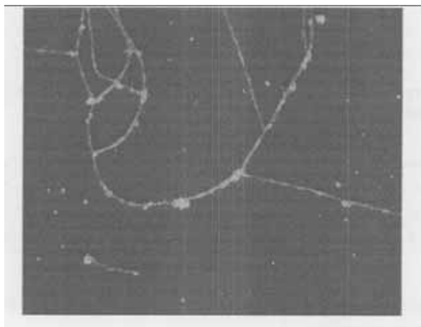
Fig. 4 Fluorescence micrograph of fibrilla morphology 16-2 deposited from aqueous solution on cover glass with magnification of 100
